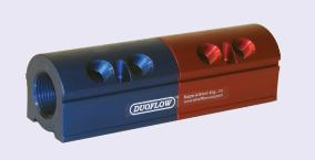
SWAP® Valves reduce time required for cooling line evacuation between mold changes to seconds instead of minutes while keeping shop floors clean. SWAP valves use shop air to evacuate fluid from cooling lines with a single handle motion.
