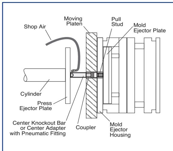
Center Bar and Coupler are installed into the Press Ejector Plate. Pull Stud is installed in the Mold Ejector Plate. Molds are changed quickly without accessing the back of the Press Ejector Plate.
