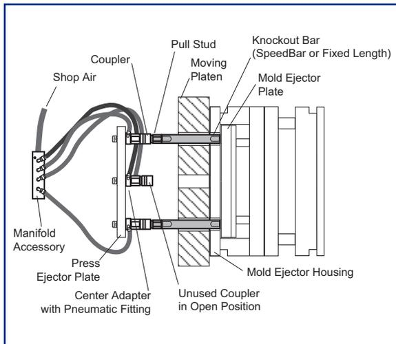
This setup is used where there is limited access to the back of the Press Ejector Plate. Custom molders using smaller presses will benefit from this application.
