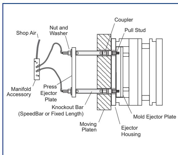
Couplers are located at the end of the knockout bars mounted to the press ejector plate.
