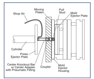
For small presses with a center knockout, replace the cylinder bolt (if present) with a Center Knockout Bar and FasTie Coupler.
