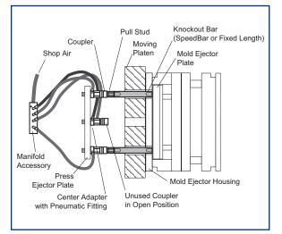
This setup is used where there is limited access to the back of the Press Ejector Plate. Custom molders using smaller presses will benefit from this application. Couplers and Center Adapters are installed on the Press Ejector Plate. Pull Studs are placed at the end of the mold-mounted knockout bars for easy removal. Molds are changed quickly without accessing the back of the Press Ejector Plate.
