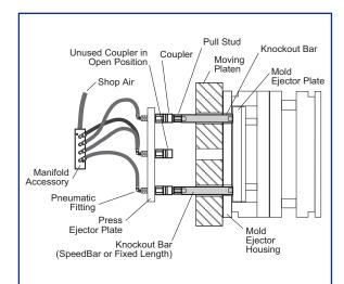
This setup is designed for custom molders who use a variety of injection molds with different knockout patterns and ejector strokes.
